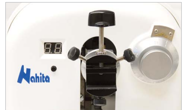
03_ Sample holder with a precise orientation system and LED counting display
