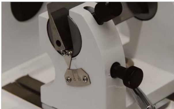
01_ Regulation system of the cutting edge angle.
