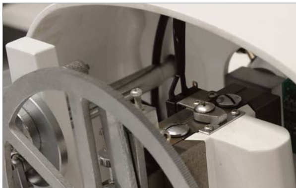
02_ It presents a locking device locks in the inner mechanism that allows holds the specimen head only in the uppermost position
