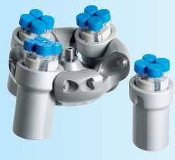
Swing-out rotor, 4-place 01324, illustrated with suspension 01398 and adapter 01483 n = 4,000 min -1 , RCF 3,305, for max. 4 x 100 ml.
