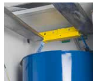
Drum gripper for forklifts to hoist 200 l drums.
