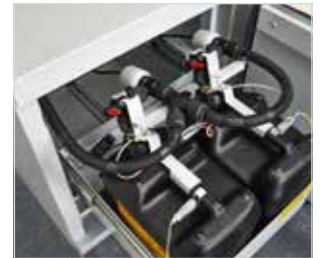
Canister changeover via an electropneumatic device, for a higher fill capacity of 20 litres.
