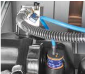
Level monitor with control module to warn about overfilling.
