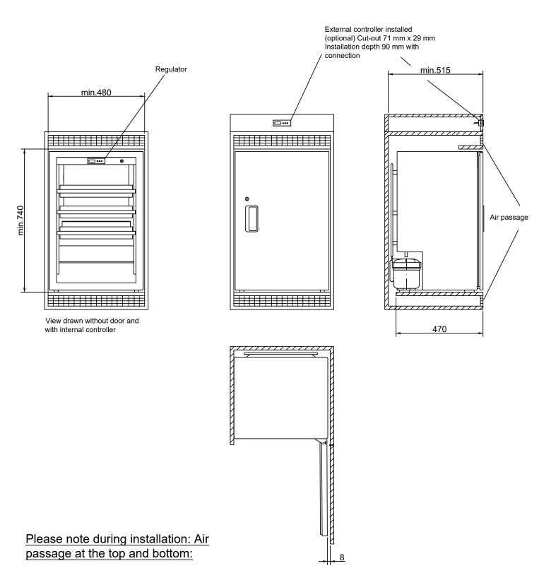
Without cooling machine fan: min. 200 cm² With cooling machine fan: min. 50 cm²
