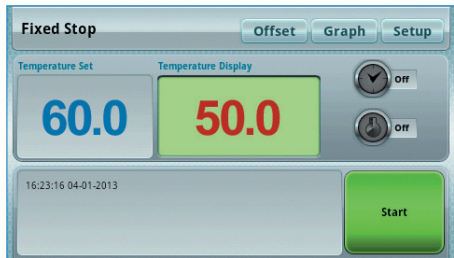
4" Full Touch Screen TFT LCD (Smart-Lab™ Controller)
