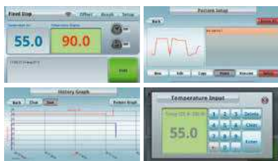
Display of Smart-Lab™ Controller
