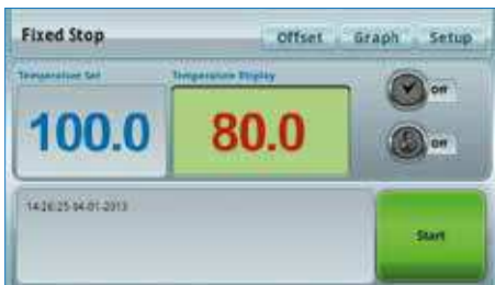
4" Full Touch Screen TFT LCD (Smart-Lab™ Controller)
