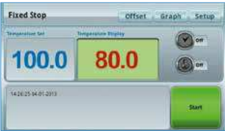
4" Full Touch Screen TFT LCD (Smart-Lab™ Controller)
